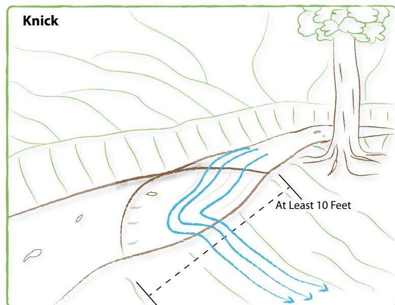
**Figure 7:** Knicks can be built into existing trails to help control water without altering the trail visibly.
