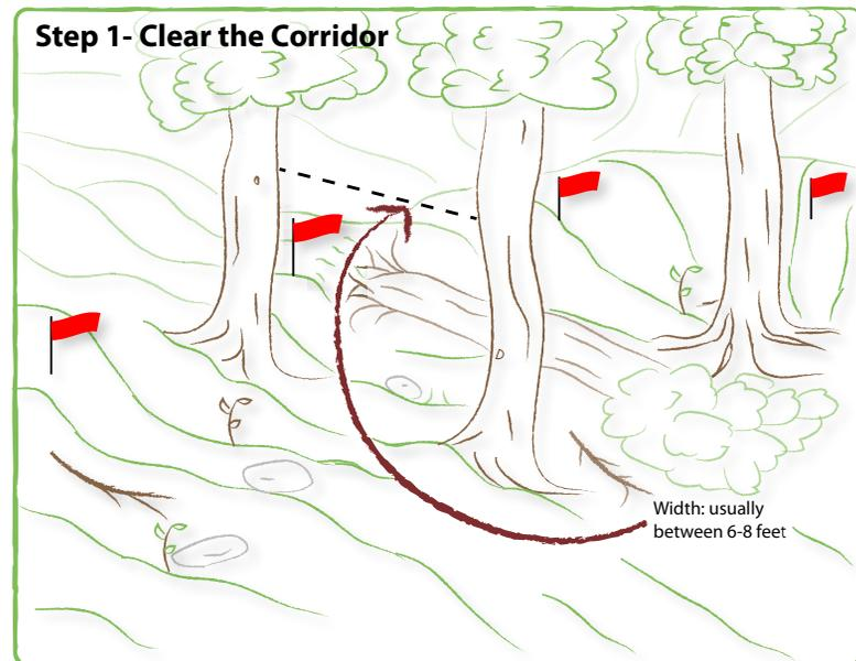
**Figure 8:** The corridor is a path 6-8 feet wide, including the tread, free of rocks, vegetation limbs and trees.
