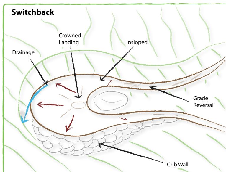
**Figure 3:** Switchbacks are turns that can help make trail more sustainable while providing easier navigation.
