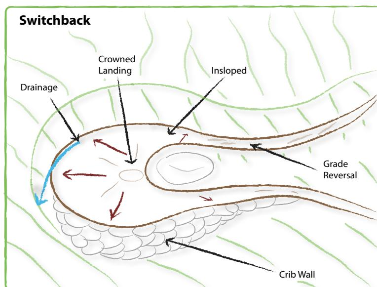
**Figure 3:** Switchbacks are turns that can help make trail more sustainable while providing easier navigation.
