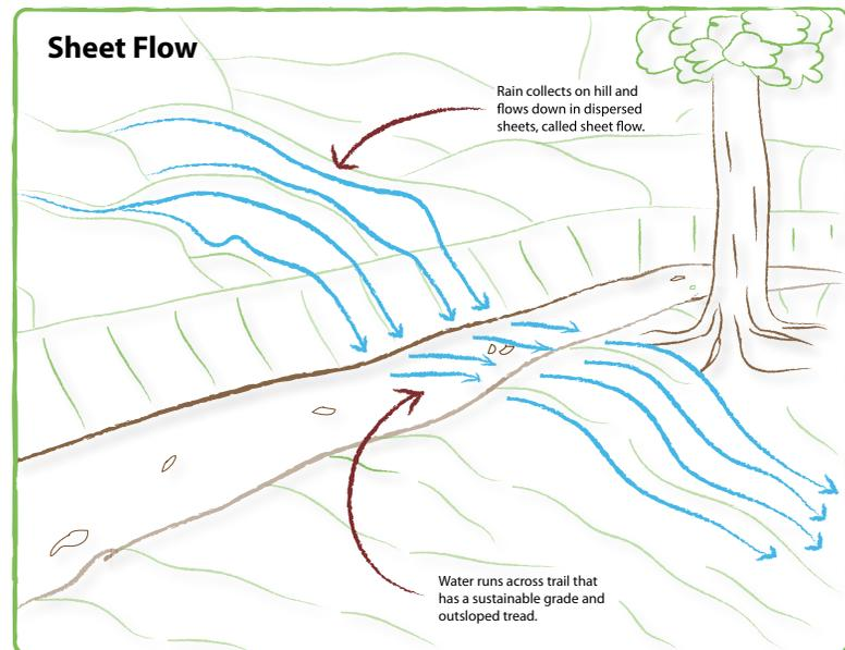
**Figure 5:** Dispersed sheets of water sheet down the cross slope and should continue across the trail for minimal damage.
