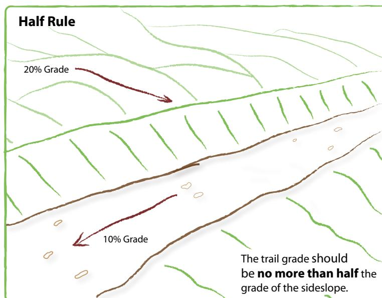
**Figure 2:** Building trail on gentle cross slopes using the Half Rule helps them to shed water.
