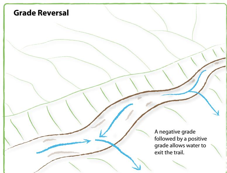
**Figure 6:** Grade reversals allow water to move off the tread at frequent intervals and should be designed into new trails.
