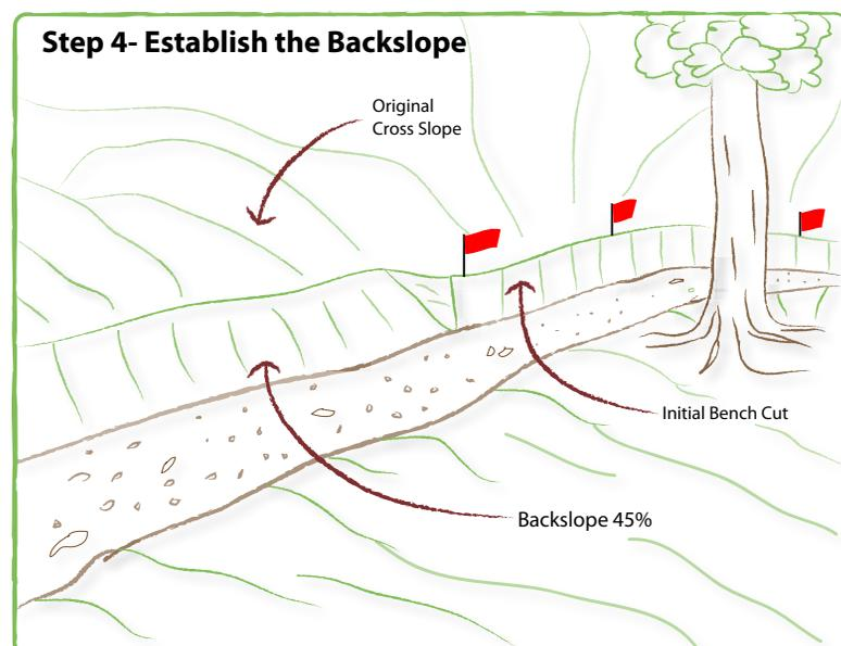
**Figure 11:** The backslope is “laid back” into the hillside as a transition between the trail and the cross slope.
