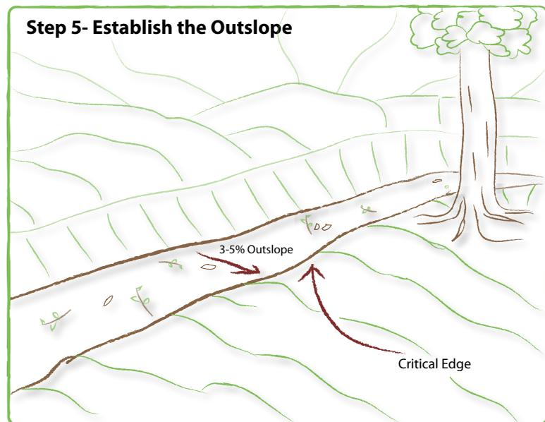
**Figure 12:** An outslope of 3-5% will allow water to continue sheeting action across the tread and over the critical edge.
