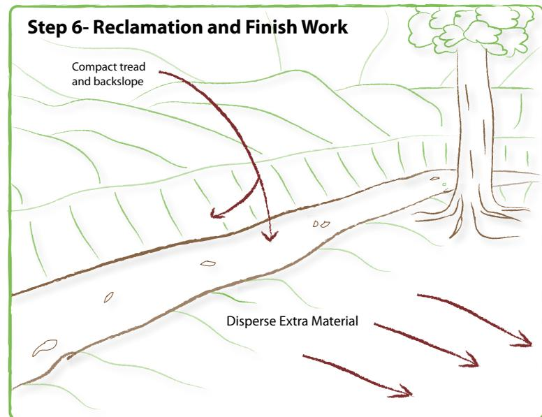
**Figure 13:** After the final step of trail building, the trail should appear as if it has always been there.
