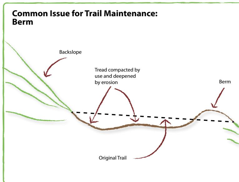
**Figure 15:** Berms on the tread prevent water from sheeting across the tread and can lead to erosion of the tread surface.
