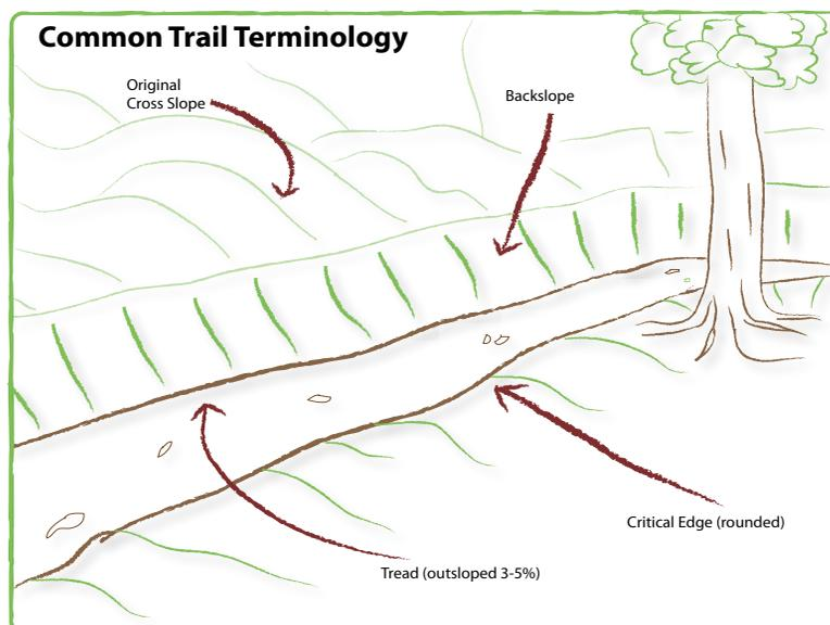
**Figure 1:** Common terms used in trail building include Cross Slope, Backslope, Tread and Critical Edge.
