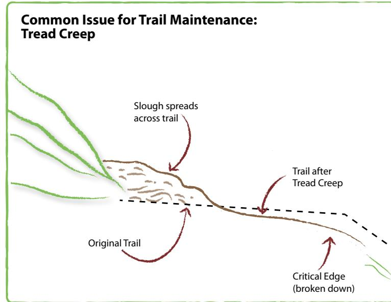
**Figure 14:** Soil rock and debris building up on the inside of the tread causes the trail to creep downhill.
