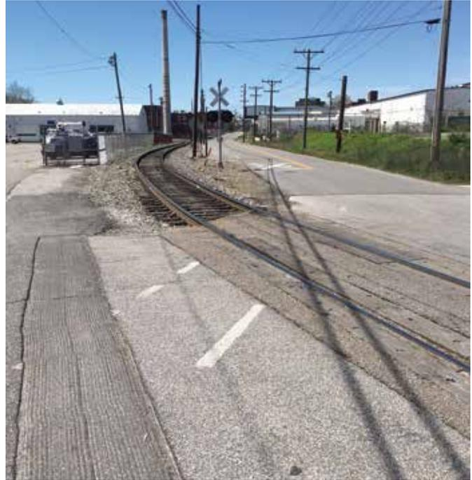
*The railroad crossing at Depot Street renders the bike lane unusable. The roadway should be widened where possible to ensure clear passing width for all users. | Photo courtesy RTC*
