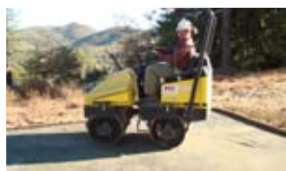
this tandem-drum walk behind vibratory roller is labor-intensive, but it produces a well-compacted product.
