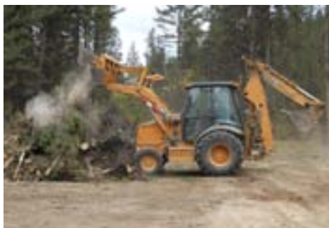
The clamshell bucket on this backhoe adds to the machine's versatility. It can scoop, load, back blade, pluck, place, and chop.
