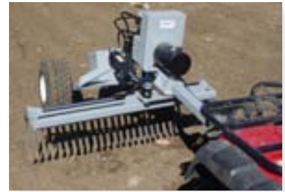
This sliding comb rake can reach out and retrieve material that is normally unrecovered and wasted in berms.
