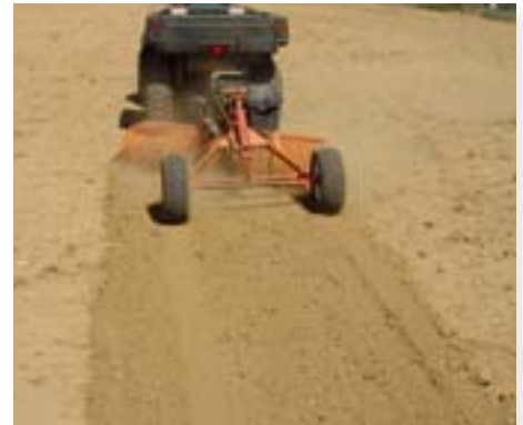
The rock rake can cut material from the edges and drift it into the center. Combs are available in different widths. At full tilt, this fixed comb extends past the width of the ATV to retrieve berms.
