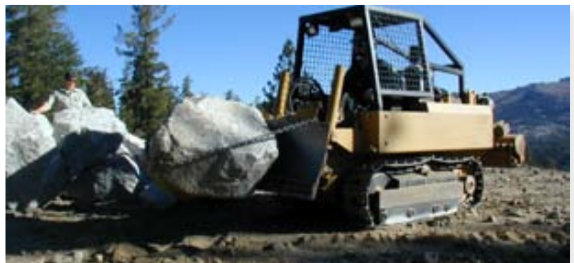
A 6-way blade makes short work of trails on steeper ground.
