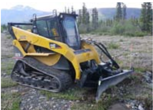
Whether used as loaders or haulers, skid steers are versatile trail-sized equipment. Because they are tracked with low center of gravity and good braking ability, they are far more stable and safer as a tow vehicle than an ATV or ROV.
