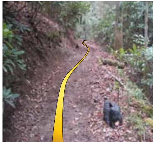
Strategically placing readily available material can produce a significant difference in the horizontal alignment.
