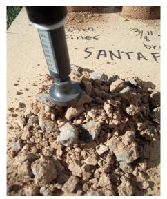
Trails on soils with fine and homogeneous textures are more erodible and often have greater potential for tread incision. Loam and sandy-loam soils, because of their even mixture of silt, clay and sand, provide the fewest limitations for trails.
