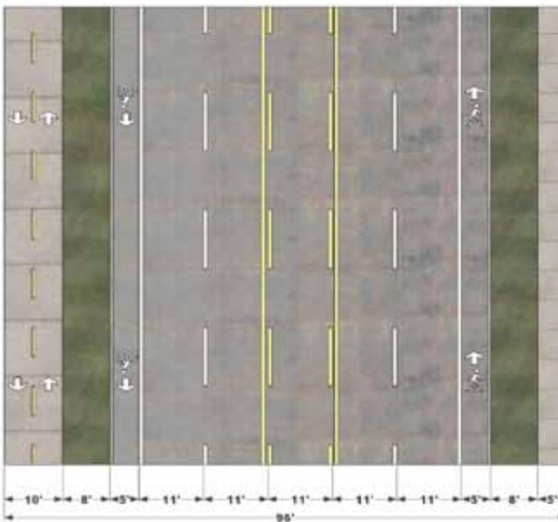
Figure 7.12. (continued) **Five-lane sections:** Top, one-way sidepaths without bike lanes; above, two-way sidepath with bike lanes
