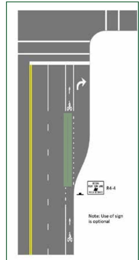
Figure 7.8. **Bike Lane Pavement Markings at RTO Lane.**
