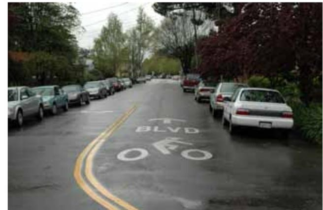
**Bicycle Boulevard.** Street modifications include special signage, pavement markings, removal of hazards like sewer grates, and traffic calming techniques. (Milvia Street, Berkeley, California)
