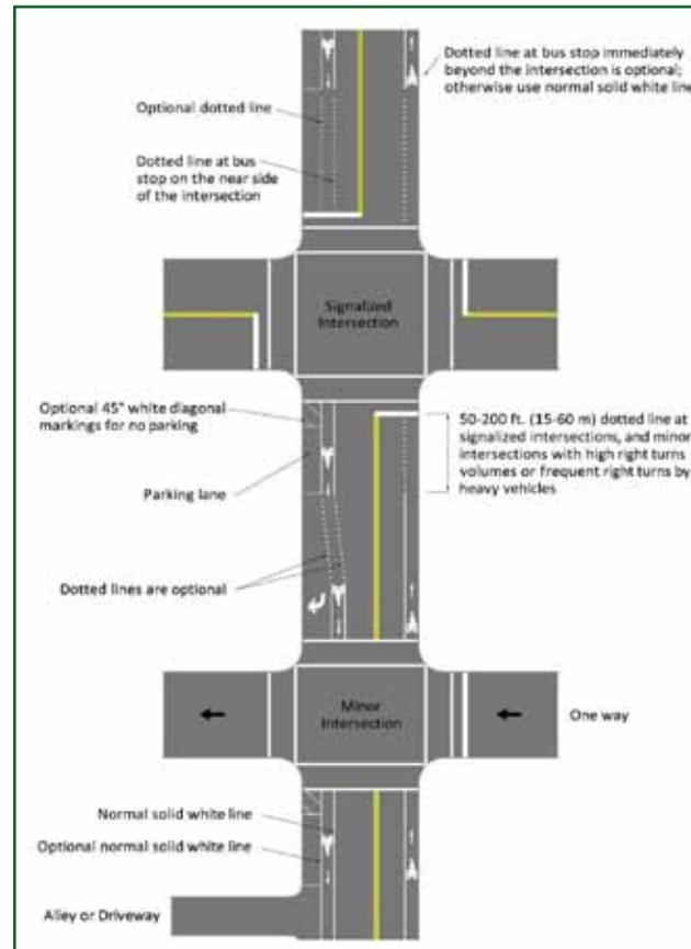
Figure 7.7. **Bike Lane Pavement Markings.**
