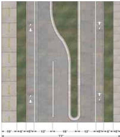
Figure 7.9. (left) **Two-lane divided section with sidepath**
