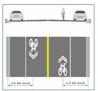
Figure 7.13. **Sharrow (shared lane marking).** Situation shown here maintains parking on both sides of the street. Source: *AASHTO 2010*
