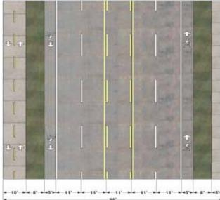
Figure 7.12. (continued) **Five-lane sections:** Top, one-way sidepaths without bike lanes; above, two-way sidepath with bike lanes
