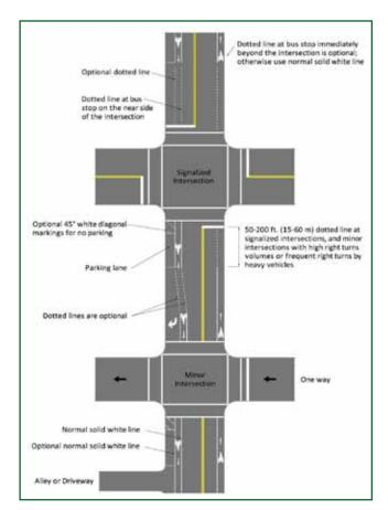
Figure 7.7. Bike Lane Pavement Markings. Source: AASHTO 2010
