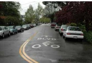
**Bicycle Boulevard.** Street modifications include special signage, pavement markings, removal of hazards like sewer grates, and traffic calming techniques. (Milvia Street, Berkeley, California)
