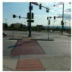
**Sidepath Intersection Design.** Principal street intersection uses a right turn median to slow right turning traffic and provide a refuge for pedestrians and bicyclists on a sidepath. (Engelwood, Colorado)
