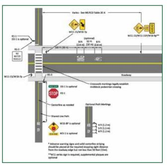
Figure 7.3. Intersection Conditions for Midblock Trail/Road Intersections: Yield and Stop Controlled Source: AASHTO 2010
