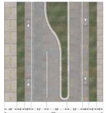
Figure 7.9. (left) **Two-lane divided section with sidepath**
