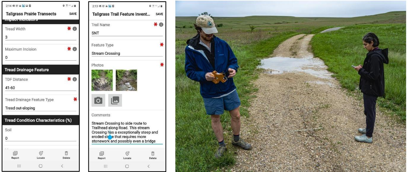
Figure 5. Examples of the Fulcrum phone app data entry forms developed for recording field data. Forms allow for the input of categorical data, metric counts or measures, text comments, and photographs.
