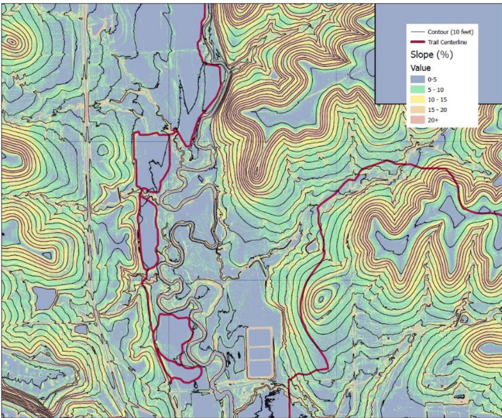
Figure 9. Slope maps with five color-coded categories showing trail system for the eastern side of the Preserve.
