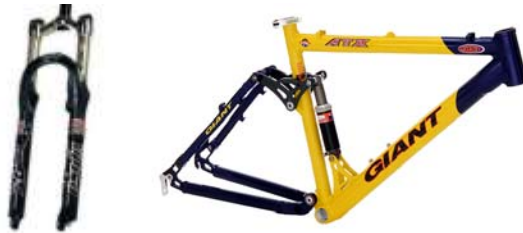
Rock Shox front suspension fork, Giant rear suspension frame
