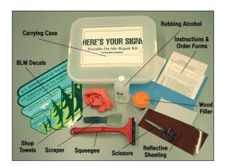
Emblems can be replaced using these tools and replacement emblems from the BLM sign kit.
