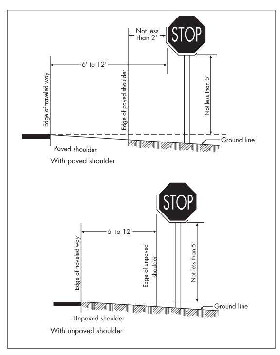
Figure 4-7. Typical Lateral Clearances and Heights.
