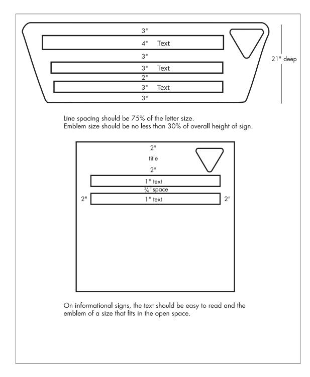
Figure 4-2. Sign Spacing and Size Guide.
