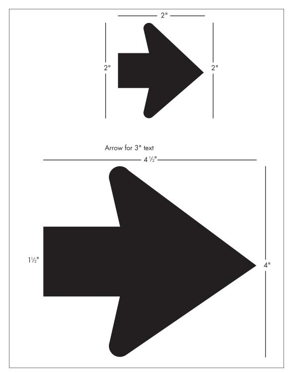
Figure 4-3. Small and Medium Arrow Sizing.
