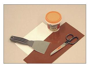
These tools from the BLM sign kit can be used to repair wood signs.
