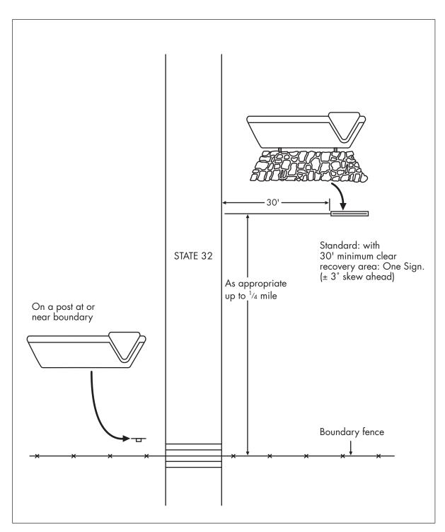
Figure 4-5. Typical Sign Installation and Properly Sized Sign Bases.
