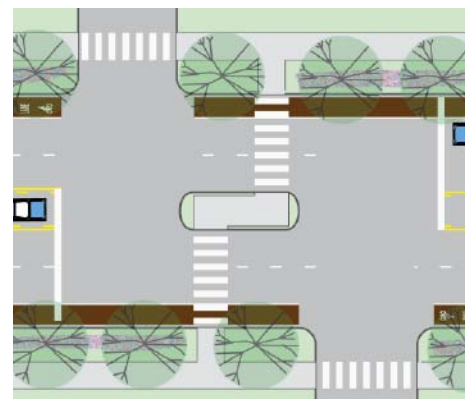
Example of a Crossing Island
