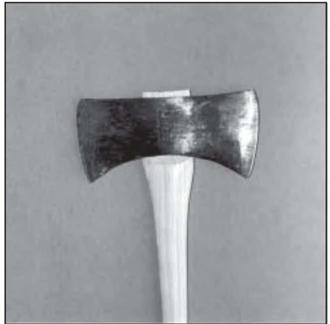
D —The tool head has been snug-fitted to the square seating shoulder. Note that there is about \frac{1}{2} inch excess handle above the head.
