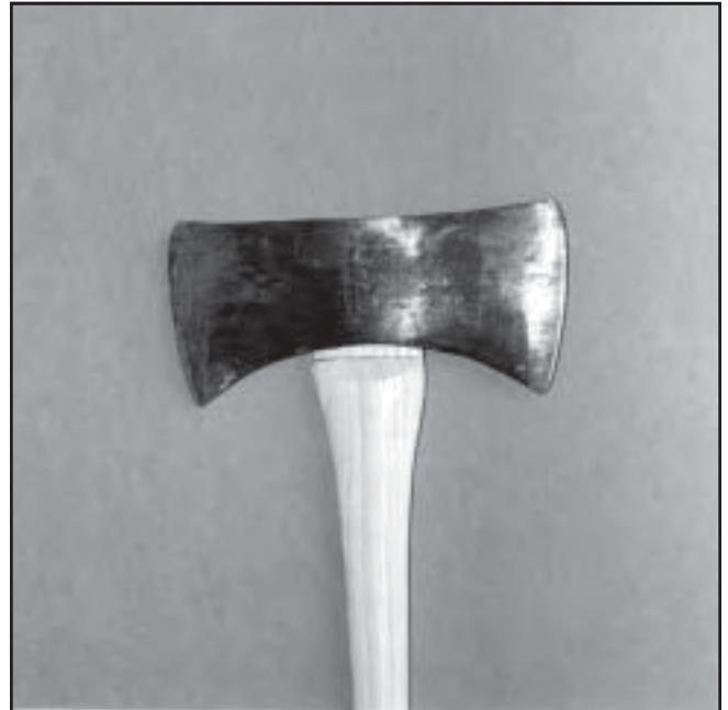
C —A line has been scribed below the roughly-fitted handle. The line denotes the final shoulder upon which the head sets.
