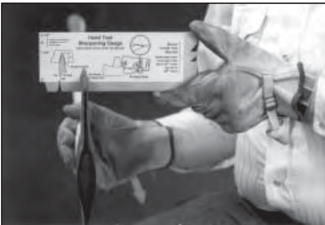
The handtool sharpening gauge is a handy aid for inspecting and sharpening a variety of fire handtools.
