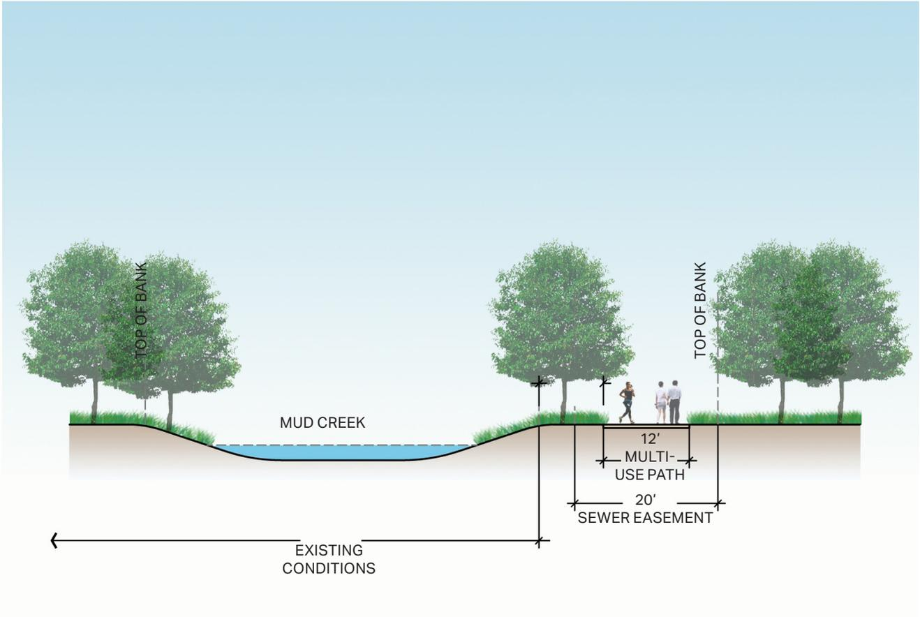
*Final design should place the trail 30 ft from the stream (outside of 30 ft stream buffer) or permits will be required.*
