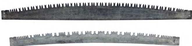
Figure 7–28. Blades of bucking (top) and felling (bottom) crosscut saws. USDA photo by Matt Able.
