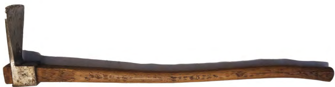
Figure 7–6. Grubbing hoe. USDA photo by Laurent Deviche.
