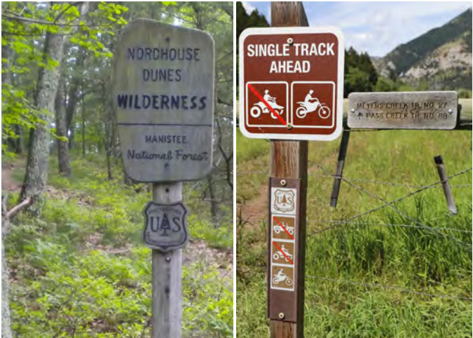
Figure 5–2. Signs in remote areas are made of wood (or material appearing like wood), similar to the image on the left. Huron–Manistee National Forests, Michigan. (USDA photo.) Signs on routes designated for motor vehicles are retroreflective as shown in the image on the right. Custer Gallatin National Forest, Montana and South Dakota. (USDA photo by Charity Parks).
