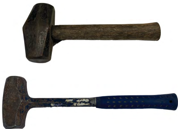
Figure 7–19. Single jack hand-drilling hammer and double jack hand-drilling hammer. USDA photo by Matt Able.
