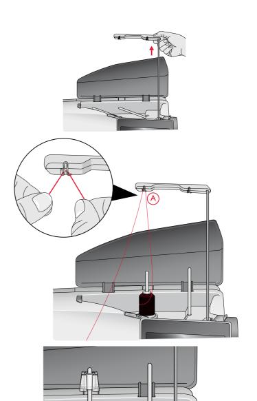
3. Hold the thread with two hands as illustrated. Floss the thread under the thread guide (A) from front to back. Pull thread back into and through threading slot (B).
