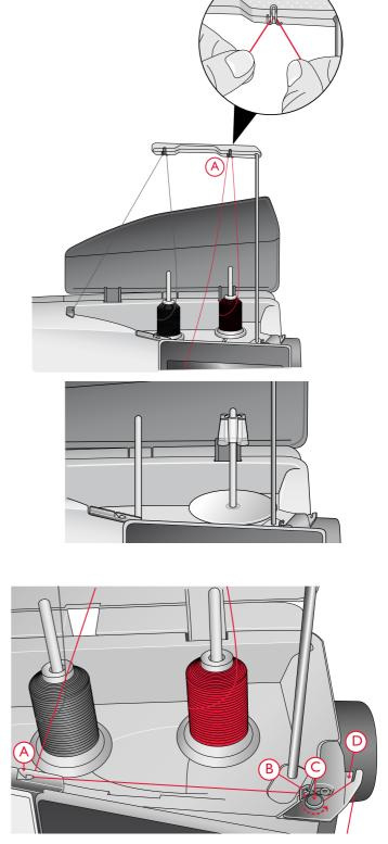
3. Place the bobbin on the bobbin spindle on the lower right side of the machine. The bobbin only fits on one way, with the logo facing out.
