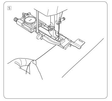
Mark the buttonhole position on the fabric and place it under the buttonhole foot. Lower the needle at the starting point by turning the hand wheel.
