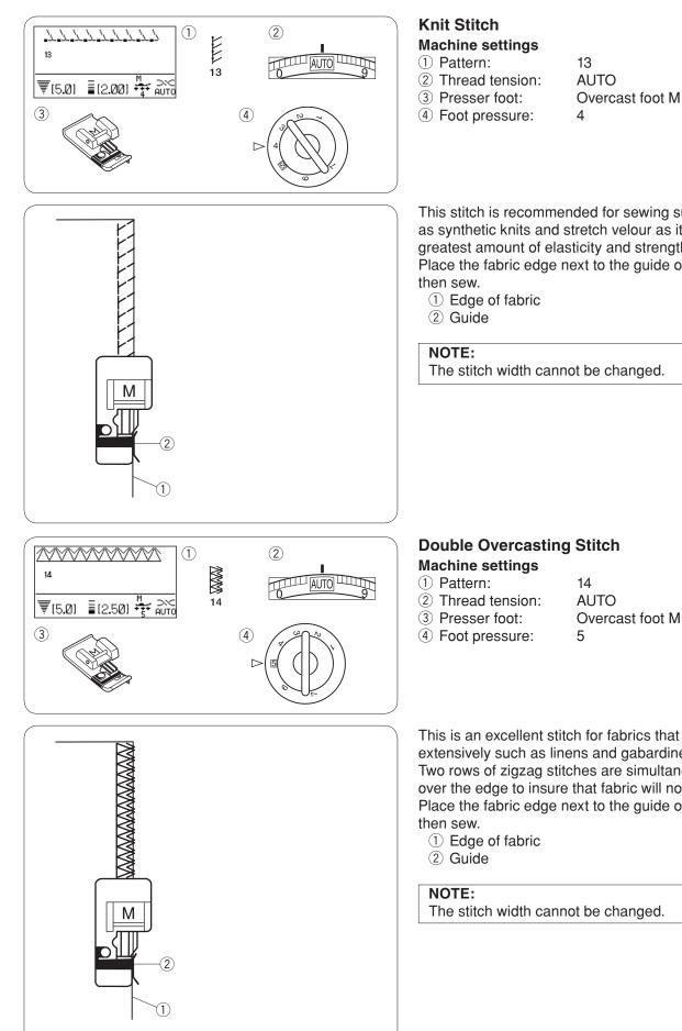
This stitch is recommended for sewing such fabrics as synthetic knits and stretch velour as it provides the greatest amount of elasticity and strength. Place the fabric edge next to the guide of the foot and
