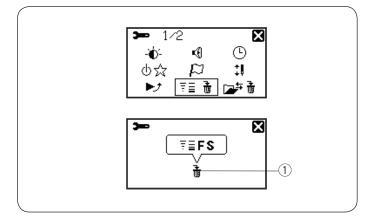
**Resetting favorite stitch length and width to default** All the customized stitch length and width settings can be reset to the original settings (factory settings).
