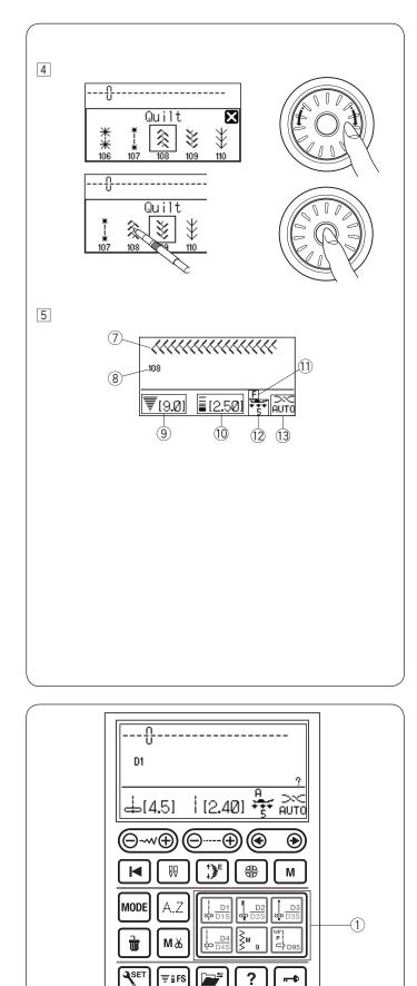
4 The pattern selection window will open. Turn the jog dial and press the confirm button, or press the stitch icon to select the desired stitch pattern.
