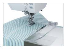
flange on the guide. Use the markings on the bed of the machine for accurate measurement and placement.
