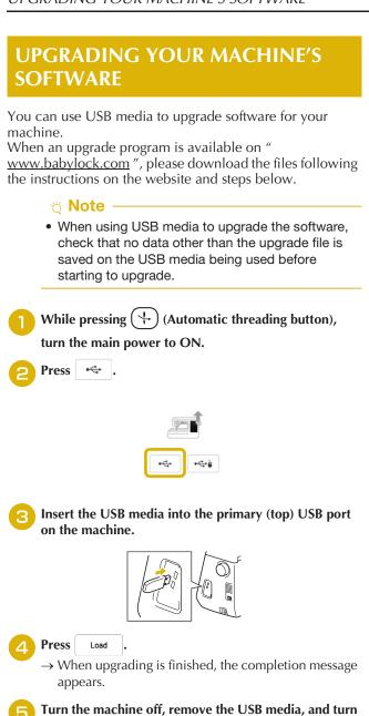
Turn the machine off, remove the USB media, and turn the machine on again.
