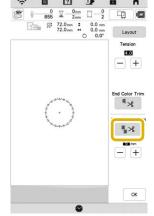
→ The key will display as  $\checkmark$ . The machine will not trim the thread before moving to the next stitching.
