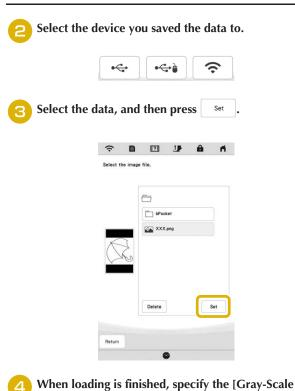
**Detection level] on the screen if necessary.** The [Gray-Scale Detection level] can change the black and white threshold for the image.
