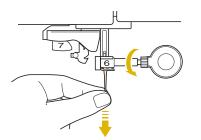
With the flat side of the needle facing the back, insert the new needle all the way to the top of the needle stopper (viewing window) in the needle clamp. Use the disc-shaped screwdriver to securely tighten the needle clamp screw.
