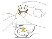
If the bobbin is inserted with the thread unwinding in the wrong direction, sewing will be done with an incorrect thread tension.
