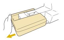
3 Slide the tab on the cover of the connection port in the direction of the arrow to open the cover.
