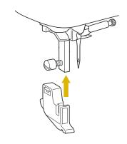
Hold the presser foot holder in place with your right hand, and then tighten the screw using the screwdriver in your left hand.
