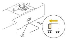
Feed dog position switch (as seen from the rear of the 1 machine)
