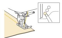
→ The machine stops with the needle in the fabric, and the presser foot is raised.
