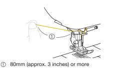
Lower the presser foot lever to lower the presser foot.
