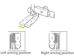
Change the needle position so that the needle does not touch the presser foot.
