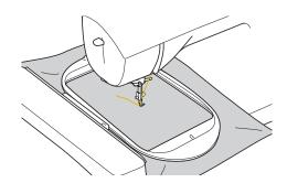
Trim the excess thread at the end of the seam. If the end of the seam is under the presser foot, raise the presser foot, then trim the excess thread.
