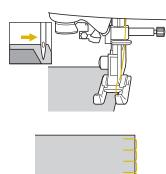
When sewing around corners, stop the machine with the needle in the fabric just outside of the appliqué, raise the presser foot lever, and then turn the fabric as needed to change the sewing direction.
