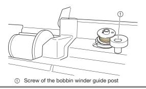
If the thread become tangled under the bobbin winder seat, press the "Start/Stop" button once to stop the bobbin winding.
