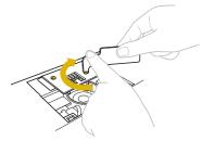
Turn the handwheel to check that the feed dogs move smoothly and do not contact the edges of the slots in the needle plate.
