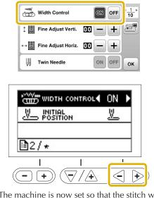
→ The machine is now set so that the stitch width can be controlled with the sewing speed controller.
