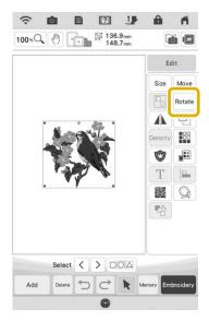
Select the key indicating the desired direction and angle for rotating the pattern.
