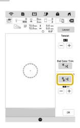
→ The key will display as  $\checkmark$ . The machine will not trim the thread before moving to the next stitching.
