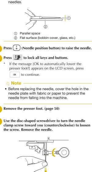
5 With the flat side of the needle facing the back, insert the new needle all the way to the top of the needle stopper (viewing window) in the needle clamp. Use the disc-shaped screwdriver to securely tighten the needle clamp screw.
