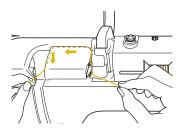
Guide the thread down, up, then down through the groove, as shown in the illustration.
