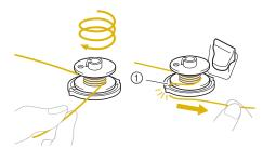
Guide slit in bobbin winder seat (with built-in cutter)
