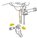
Set the adapter on the presser foot bar, aligning the flat side of the adapter opening with the flat side of the presser bar. Push it up as far as possible, and then tighten the screw securely with the disc-shaped screwdriver.
