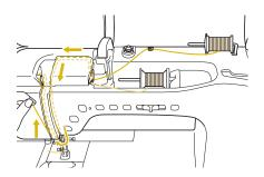
Continue threading; however, do not pass the thread in the needle bar thread guide "6" on the needle bar. Thread the needle on the right side.
