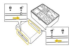
Place the lid on top of the case so that the notches in the lid align with the tabs on the case, and then slide the bar on each side back to the locked position.
