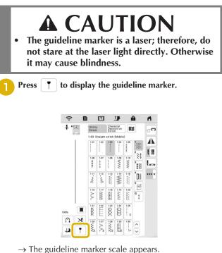
Depending on the setting of "Initial Position" in the settings screen, the initial needle drop point is scaled as either 0.0 mm or 3.5 mm.
