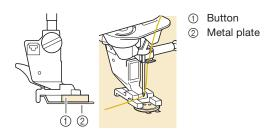
Rotate the handwheel toward you (counterclockwise) to check that the needle goes into each hole correctly.
