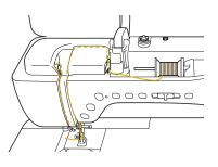
Pass the thread through the needle bar thread guides on the needle bar, then thread the needle on the left side manually.
