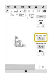
→ The key will display as <a>></a>. When one color thread is embroidered, the machine will stop without cutting the thread.
