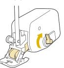
When the feed position lever is down, the black roller belt on the dual feed is engaged.
