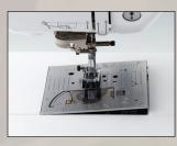
**One Action Needle Plate** Allows for quick needle plate changes without the use of a screwdriver. No need to remove your extension table, embroidery unit or accessory tray.
