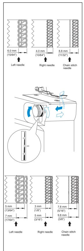
Use of width adjustment dial will permit further adjustment within the width range shown below.
