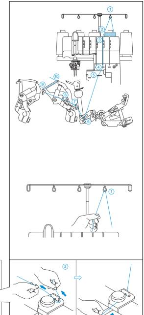
(2) Thread the top cover thread guide by pulling the thread towards the left until it slips under guide. Then pull thread along the right side of pretension disc as illustrated. ③ While holding thread with finger, pass it between the tension discs and pull thread down to make certain it is properly located in between the tension discs.
