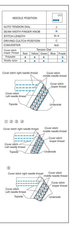
① Since the seams formed by cover stitch unravel when the looper thread is pulled out at the end of sewing, secure the seam end in the following manner.
