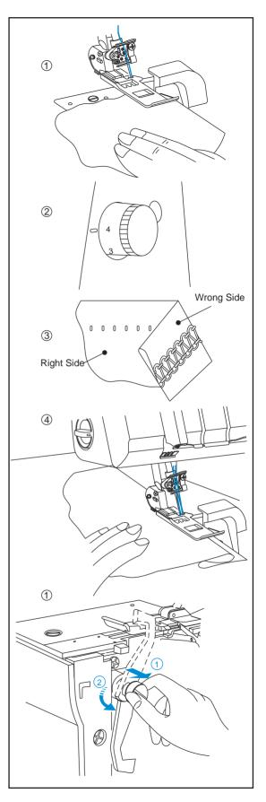
(2) Fold the fabric with the wrong sides together. Sew with the stitches lying neatly on the edge of the fold.
