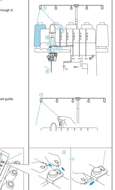
② Thread the top cover thread guide by pulling the thread towards the left until it slips under guide. Then pull thread along the right side of pretension disc as illustrated. ③ While holding thread with finger, pass it between the tension discs and pull thread down to make certain it is properly located in between the tension discs.
