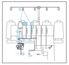
① Pass thread from back to the front through thread guide.
