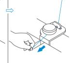
(3) While holding thread with finger, pass it between the tension discs and pull thread down to make certain it is properly located in between the tension discs.
