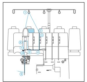
(1) Pass thread from back to the front through thread guide 1.
