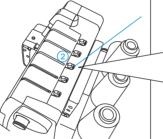
③ While holding thread with fingers, pass it between the tension discs and pull thread down to make certain it is properly located in between the tension discs.
