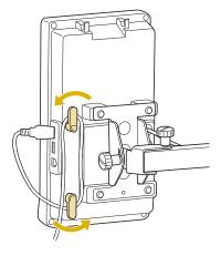
Insert the card completely into the card reader/USB card writer module\*.
