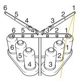
Place on spool pin 1 the spool of thread with the color (lime green) specified for needle bar 1.
