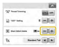
A value between 0 and 1 millimeters if the units of measurements is set to "mm" (or a value between 0 and 0.04 inch if the units of measurements is set to "inch") can be specified.
