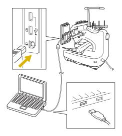
If the machine is positioned at a distance that the USB cable does not reach the computer, embroidery patterns can be transferred from the computer by temporarily saving them on USB media, which is then connected to the machine. Refer to "USB media" on page 158.
