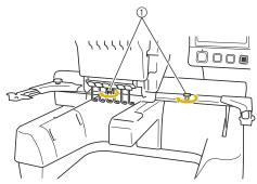
① Use the thumb screws included with the machine (thumb screws removed in step 1) on page 225).
