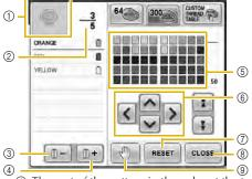
① The part of the pattern in the color at the top of the thread color sequence display is the part whose color is being changed.
