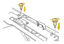
While pushing in the cap frame driver toward the machine so that it is fully inserted, tighten the two lower thumb screws to secure the cap frame driver.
