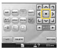
The pattern can also be moved by dragging it. If a USB mouse is connected, move the mouse to position the pointer on the desired pattern, and then hold in the left mouse button while dragging the pattern. The pattern can also be dragged by selecting it directly in the screen with your finger or the touch pen.
