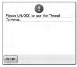
The thread trimming button was pressed before the machine was unlocked.
