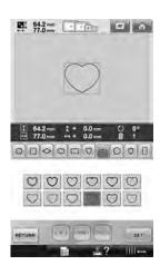
Select a frame pattern sewn with straight stitches to embroider onto the fabric for the appliqué. Carefully cut outside of the stitching.
