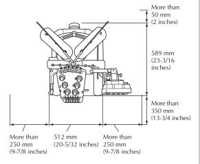
Adjust the legs so that the machine is steady.
