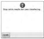
The machine was stopped while the needle bar case was moving.
