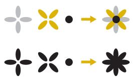
In order for the parts of the pattern to be differentiated when Tajima data is used with this machine, the pattern is displayed with colors automatically applied in the default thread color sequence. Since the thread colors are applied according to the sewing order of the parts, regardless of the design of the pattern, colors may be applied that seem unusual for the design, for example, an orange-colored fruit may be displayed in blue.
