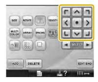
► The pattern moves in the direction of the arrow on the key.
