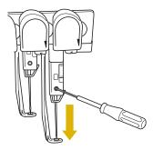
► The needle and presser foot are locked in the down position.
