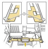
① Make sure that the pins on the left and right arms of the embroidery frame holder fit into the positioning slot and hole on the embroidery frame.
