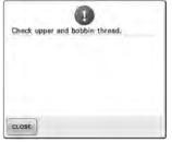
The upper thread broke, the thread came out of the thread tension disc or a thread guide, or the machine is not threaded correctly.
