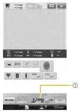
① Shows the amount of free space in the USB area of the machine. If pattern data with this size is added, it can be recalled (temporarily written).
