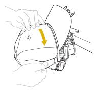
Use the clips to secure the cap.
