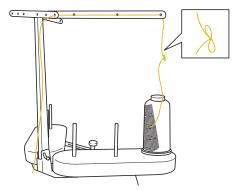
Pull out the old thread just after the needle bar thread guide.
