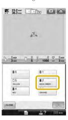
Touch the number of the other needle bar that will be switched. The two needle numbers are connected with an arrow.
