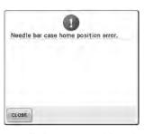
The needle bar case could not be moved to its initial position.
