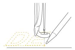
Remove the embroidery frame from the machine, and then connect these two points to check the embroidering position.
