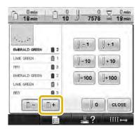
Each time this key is touched, the next color in the thread color sequence display is selected. After reaching the last color in the thread color sequence display, the first color is selected.
