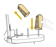
Tie the end of the thread on the new spool with the end of the thread remaining from the previous color.
