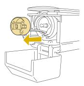
Rotate the handwheel (about 50 degrees) to move the race of the hook to a position where it can easily be oiled.
