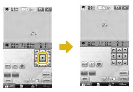
The pattern can also be moved by dragging it. If a USB mouse is connected, move the mouse to position the pointer on the desired pattern, and then while holding in the left mouse button, drag the pattern. The pattern can also be dragged by selecting it directly in the screen with your finger or the touch pen.
