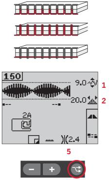
*Press the alternatives button to view stitch positioning and density*
