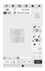
Using the included touch pen (stylus), touch  $\checkmark$ , and then draw lines to trace the image.
