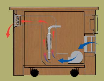
With SewComfort Heaters, air is drawn from the floor level through a washable lifetime filter. This filtered air then enters the heating chamber, passes through an exclusive mineral-filled tubular heating element, and then out of the heater through a specially-designed front louvered grill.
