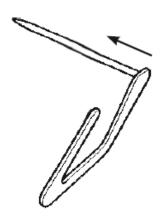
2. Adjust the stem of the quilt bar so that the guide aligns with the seam that has already been sewn.
