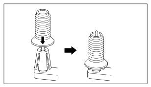
When using thread on cones, place the cone over the cone holders on the spool pin.
