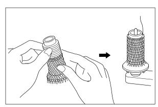
Thread spool nets are useful for synthetic threads which tend to drop off its holder.
