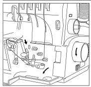
Open the front cover and rotate the handwheel to bring the upper looper to its lowest position.
