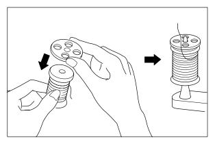
Thread caps are also provided with the accessories. They are used when sewing with regular spools. Insert the stem of cap into the spool hole opposite the end with notch.
