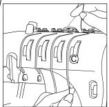
C. Bring thread straight down along the slot so that the thread passes between the tension discs.
