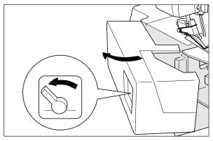
Swing Extension Table out with lever in locked position and Free Arm Cover will stay attached to the Extension Table.
