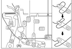
3. Remove the lower looper thread from the thread guide (A).
