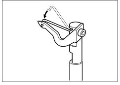
Push on the subsidiary looper with your finger and rotate it to the left until the tip of the subsidiary looper is securely positioned into the eye of the upper looper.
