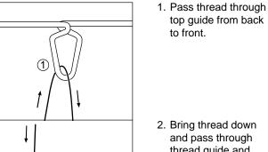
2. Bring thread down and pass through thread guide and under pretension disc.
