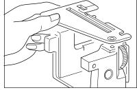
7. Lift the Needle Plate off and replace with Rolled Hemming Plate. (Be sure that thread is not caught under plate.)
