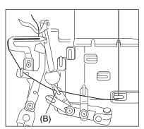
4. Hook the lower looper thread to the thread guide (B).
