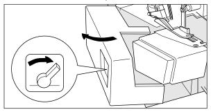
Turn lever located on left side of extension table to the front of machine and swing table out.
