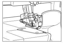
8. Retighten the screw and replace Free Arm Cover.
