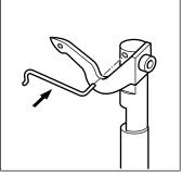
5. Insert the subsidiary looper into the hole at the top of the upper looper shaft.
