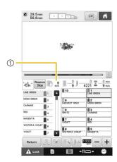
① Time until the machine stops
