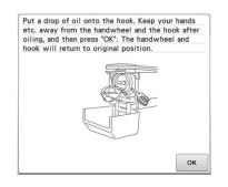
After oiling, insert the bobbin case into the hook, and then close the hook cover. (Refer to page 37.)
