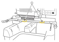
Use the thumb screws included with the machine (thumb screws removed in step 1 on page 262).
