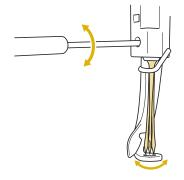
**3** With the flat side of the needle toward the back of the machine, insert the needle all the way up until it touches the needle bar stopper.
