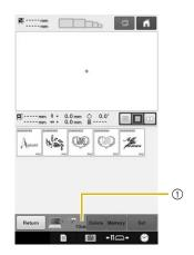
① Shows the amount of free space in the USB area of the machine. If pattern data with this size is added, it can be recalled (temporarily written).
