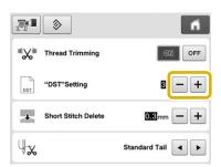
• A value between 1 and 8 can be specified. For example, if 3 is specified, sequential 3 jump codes will be converted to the trim code. But sequential 2 jump codes will not be converted to the trim code, it will be sewed as the feed (jump) stitch.
