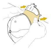
**15** While pulling the lever toward you that is located behind the handle on the right side of the mounting jig, rotate the cap frame to the left. After the cap frame has been rotated 90°, release the lever to lock the cap frame in place.
