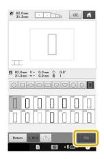
Before embroidering, touch **to** display the pattern connection setting screen. In this example, we will select the top point of the right edge for the second pattern.
