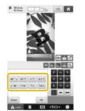
• Touch the positioning keys to move the embroidery frame until the pattern in the camera view window is aligned with the chalk mark drawn on the fabric.
