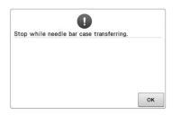
The machine was stopped while the needle bar case was moving.
