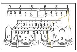
Pass the thread of a specified color through the holes on the thread guide, making sure that you have the thread color matched to the coordinating needle bar.
