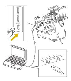
If the machine is positioned at a distance that prevents the USB cable from reaching the computer, embroidery patterns can be transferred from the computer by temporarily saving them on USB media or an SD card, which is then inserted into the machine. (Refer to "Saving embroidery patterns to USB media/SD card" on page 160.)
