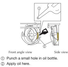
• Use a pointed object to punch a small hole in the tip of the included oiler before using it.
