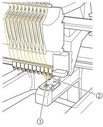
Needle hole in the needle plate
