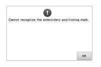
Machine failed to recognize the embroidery positioning mark. Confirm that the embroidery positioning mark is in the selected area. If problem persists, reposition the mark.
