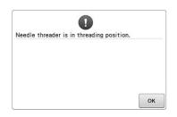
Another operation was performed while the automatic needle-threading mechanism was threading the needle. Press the automatic needle threading button, and then perform the other operation after the needle is threaded. (Refer to page 61.)
