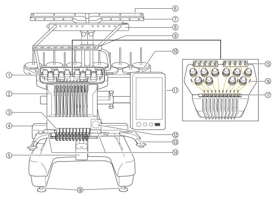
① Thread tension knobs
