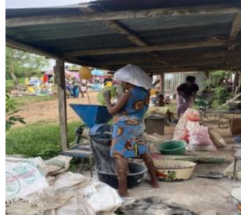
Milling dried plantain flakes into flour with plate attrition mill, Nigeria
