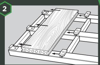
Place the first piece of decking on the timber frame with the decking running perpendicular to the joists. The first piece of deck may be secured with starter clips. **Do not screw or nail through** *HD Deck® Dual*, use 1 clip and screw on every joist.
