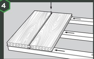
Take the next piece of deck and securely push into the clips. Now nip the screw to secure the clip against the board. **Do not over tighten**.
