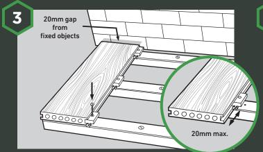
Take a screw, place in the hole located in the clip and screw into the wooden joist. Do not tighten at this stage. Make sure the boards **do not** over hang the joist at the edge by **more than 20mm** and a **20mm expansion gap** should be left between the wall or other fixed objects surrounding the deck.
