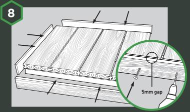
Drill pilot holes with counterbore through the fascia at 200mm - 300mm intervals. According to ambient temperature allow a **5 - 7mm gap** between end of deck board and the fascia. Screw fascia to the joist. Always screw fascia to the joist at a 90° degree angle.
