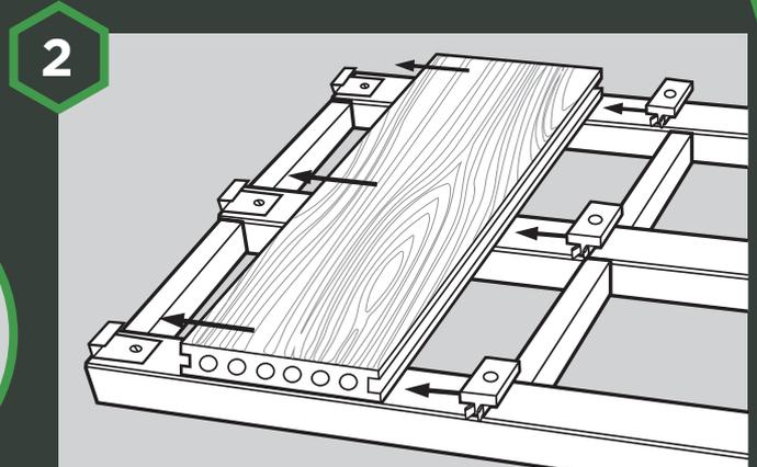
Place the first piece of decking on the timber frame with the decking running perpendicular to the joists. The first piece of deck may be secured with starter clips. **Do not screw or nail through HD Deck® Dual**, use 1 clip and screw on every joist.
