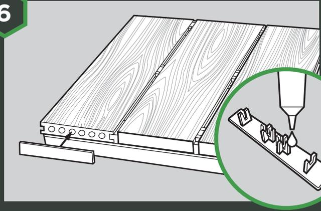
If using end caps, apply a high quality grab adhesive to the end caps to secure for extra adhesion. Wipe away any excess from the edge of the cap.
