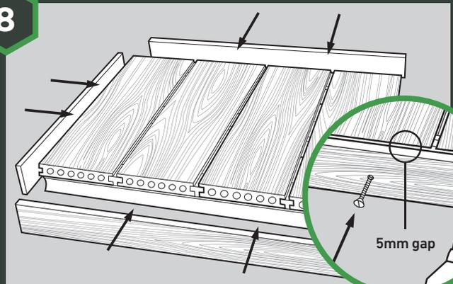
Drill pilot holes with counterbore through the fascia at 200mm - 300mm intervals. According to ambient temperature allow a **5 - 7mm gap** between end of deck board and the fascia. Screw fascia to the joist. Always screw fascia to the joist at a 90° degree angle.
