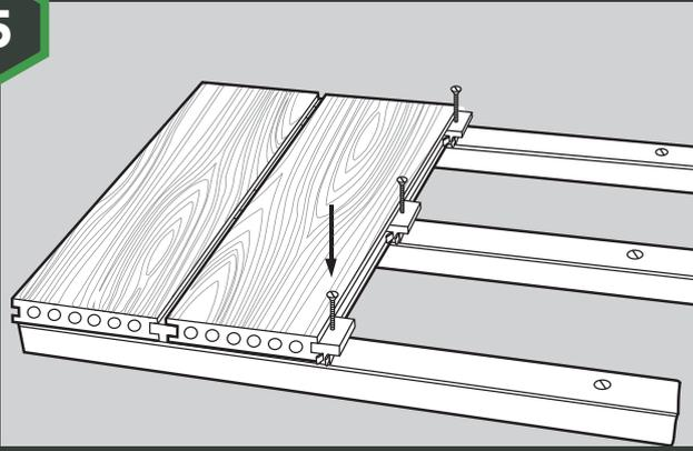
Now repeat steps 3 and 4 to cover the deck, using 1 clip and screw on every joist.
