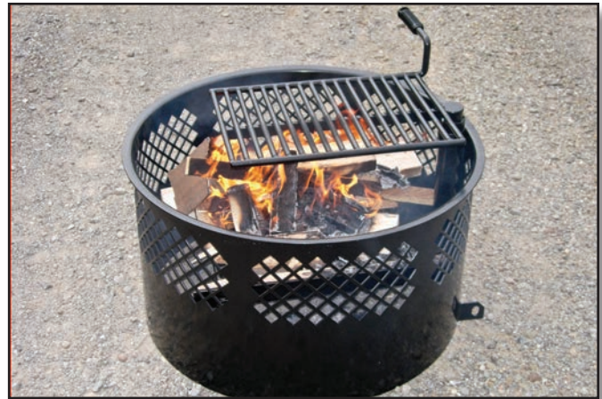
Figure 86—This manufactured fire ring has an internal grate that elevates the fire-building surface 9 inches (230 millimeters) above the ground. The mesh ring above the fire-building grate allows enjoyment of the fire and allows air supply to aid combustion. The cooking grate swings to the side for access to the fire. Photo credit: Jamestown Advanced Products Corporation, Jamestown, NY
