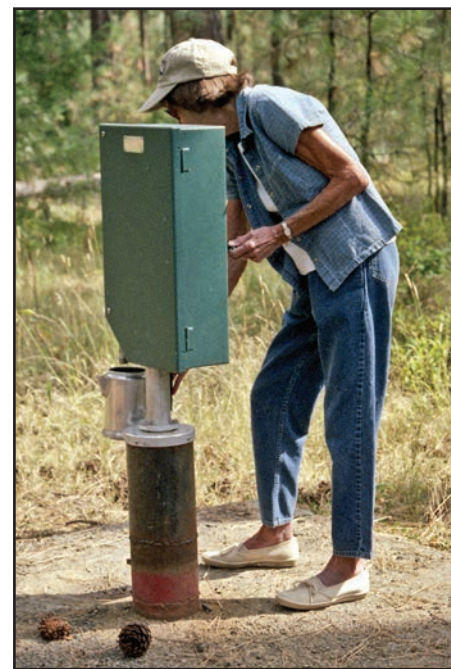
Figure 102—An accessible handpump developed by the Missoula Technology and Development Center.
