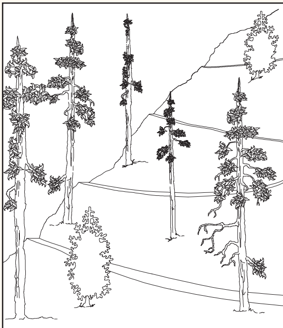
Figure 121—A trail with a 5-percent grade on a steep hill.
