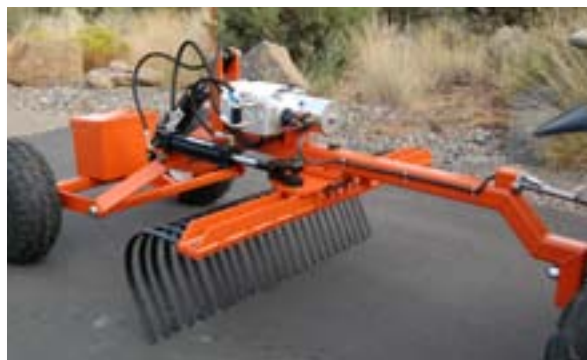
This fixed-comb rock rake has hydraulic rams which have proven durability in dusty conditions. The steel tines are replaceable. Which ones wear out first? The outer ones since most trails are cupped by the forces of compaction and displacement.
