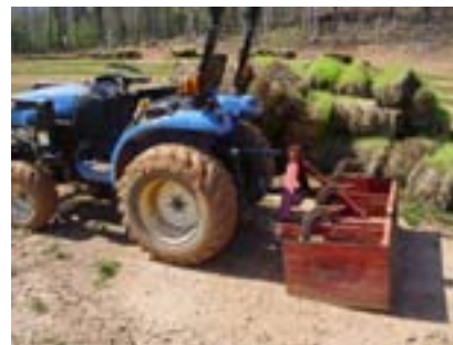
Box blades have ripper teeth inside the box, which shapes and compacts the material.
