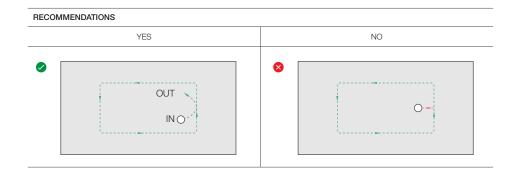
To do large cutouts or large parts, you must remember the following cutting sequence.
