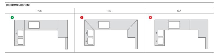
An empty space of at least 3 mm that functions as an expansion joint must be provided between the product and the wall against which it is rested, for seaming 2 mm between the pieces is recommended.
