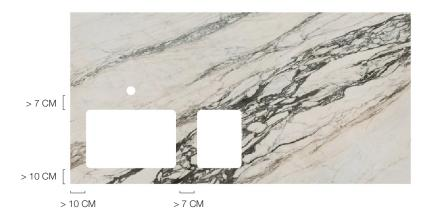
Flush-mount housing and cut-outs for the elements to be flush-mounted (sinks, cook tops, etc.) must provide an additional perimeter space of about 1.5mm that functions as an expansion joint.
