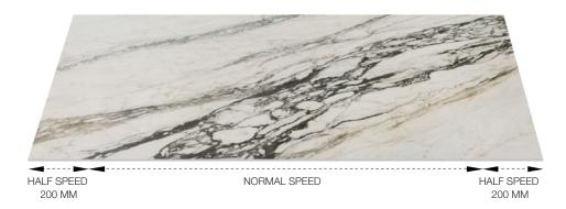
In general, the feed rate must be reduced depending on the cut's complexity, the slab's thickness, and the disc's technical features. That's why we recommend machines that allow for adjusting their RPMs as well as their feed rate.
