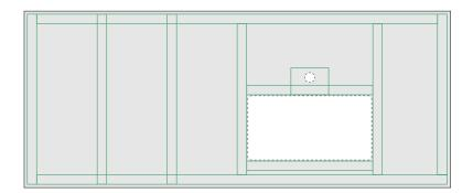
Arrange the structure of the cabinets being covered so that it is level, stable, clean and suitable to receive the weight of the countertop. The structure of the furniture must be checked periodically in terms of levelling, compensating for any misalignments.
