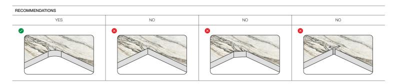
Joints between slabs and other materials whenever these slabs are combined with other surfaces (e.g. furnishings, walls, metal accessories, window fixtures) require elastic grouting, it's important to define the distance between them, taking the following into account:
