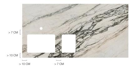
Flush-mount housing and cut-outs for the elements to be flush-mounted (sinks, cook tops, etc.) must provide an additional perimeter space of about 1.5mm that functions as an expansion joint.
