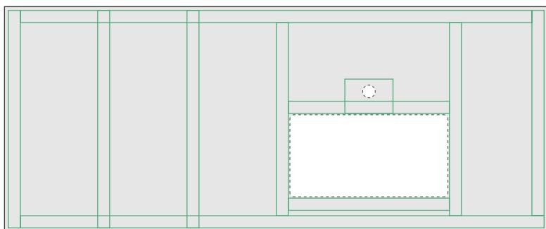
Arrange the structure of the cabinets being covered so that it is level, stable, clean and suitable to receive the weight of the countertop. The structure of the furniture must be checked periodically in terms of levelling, compensating for any misalignments.
