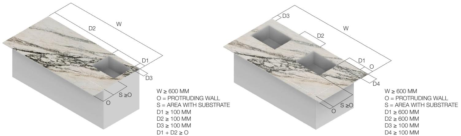
For standard lengths that exceed an overhang of 30 cm, an adequate support must be provided from the bases, at least every 60 - 62 cm.
