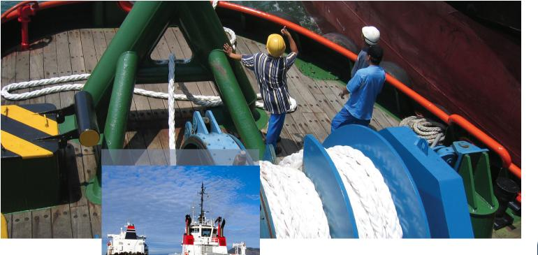
SWOS implements patented technology that permanently increases the coefficient of friction of these ropes so that they grip much better on bitts, and provides a much longer lasting product in this rigorous application.
