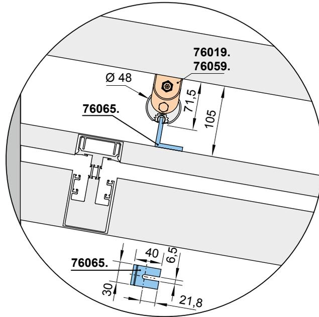
03 Support to prevent deflection of the cover support tube, can be shortened on site, height range 70–320 mm
