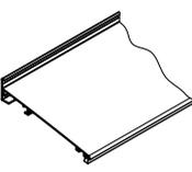
Wall sealing profile incl. brush seal when installing with a coverboard
