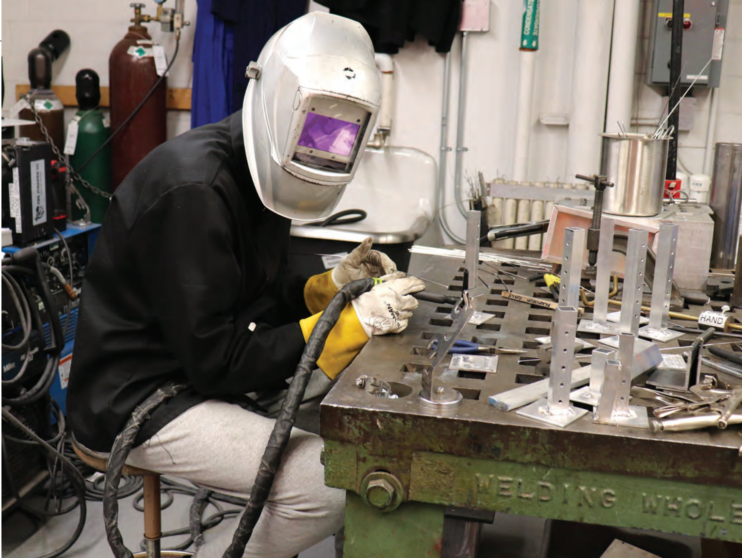
▲ Joseph Harrington Th'24 practices tungsten inert gas, or TIG, welding aluminum in the Machine Shop. Photo by Tishya Khanna Th'24
