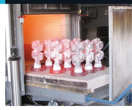
other good way to remove wax if the autoclave failed. Another challenge was scheduling in the foundry due to burnout capacity and timing.
