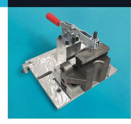
downtime of the production order associated with tooling work. The picture above shows the fixture built at TPM with the appropriate casting inserted.
