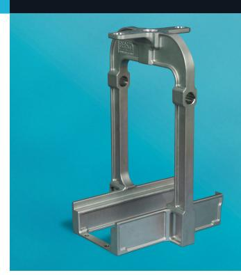
pockets were added to make the cast as light as possible, while still maintaining the strength needed for utilization. Branding was also incorporated into the casting design.
