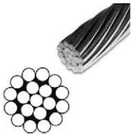
Stainless Steel 316 Cable Ø3/16", 1X19 Construction
