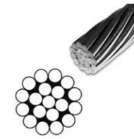
Stainless Steel 316 Cable Ø3/16", 1X19 Construction
