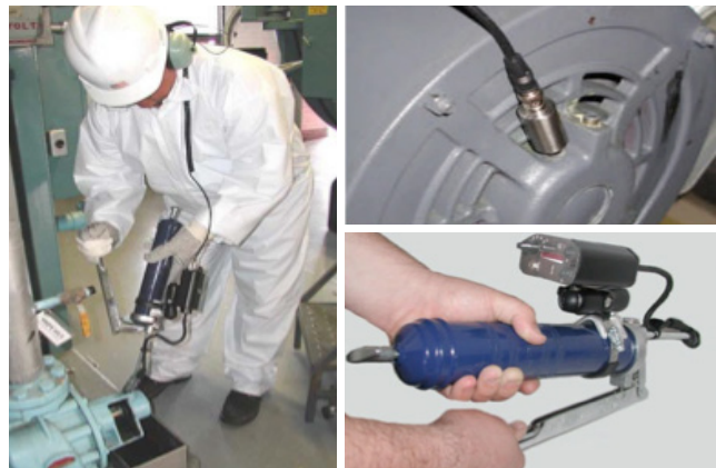
Figure 7. Ultrasonic Assisted Lubrication
